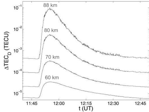
**Fig. 4.** Time evolution of  $\Delta\text{TEC}_D$  in layers (of thickness of 2 km) located at altitudes 60 km, 70 km, 80 km, and 88 km during the considered solar X-ray flare.
