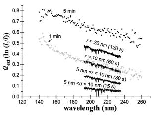
Fig. 2. Extinction curves  $(Q_{ext})$  for different particle radii (different discharge times). UV extinction curves are measured with two different spectrographs/detecting systems: solid lines - extinction measured with UV/VIS spectrograph and ICCD; solid circles and opened triangles - extinction curves for extended spectral region (VUV).
