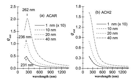
Fig. 3. Extinction curves for different particle radii. The refraction index necessary for the calculation of  $Q_{ext}$  was taken from Zubko et al. (1996): (a) low-hydrogenized material, graphitic-like (ACAR); (b) hydrogen-rich material, polimer-like (ACH2).
