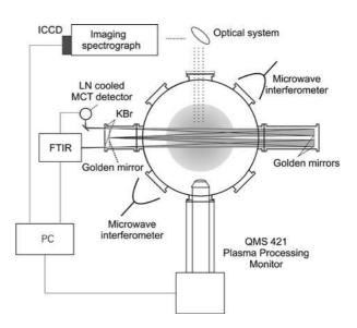
**Fig. 1.** Experimental set-up, top view. For the more detailed explanation and abbreviations see text.
