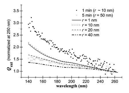
Fig. 4. Comparison of calculated and measured UV extinction curves for different particle radius: solid lines - calculated curves for ACH2 material according to Bohren and Huffman (1983) with  $Q_{ext}$  from Zubko et al. (1996); symbols - measurement results.
